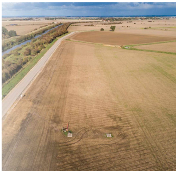
Image 5.16 Typical reinstatement of an open cut swathe with two joint bays (Source: Murphy Group, 2019)
